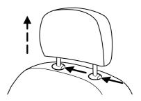
To reinstall the adjustable head restraint, do the following:
